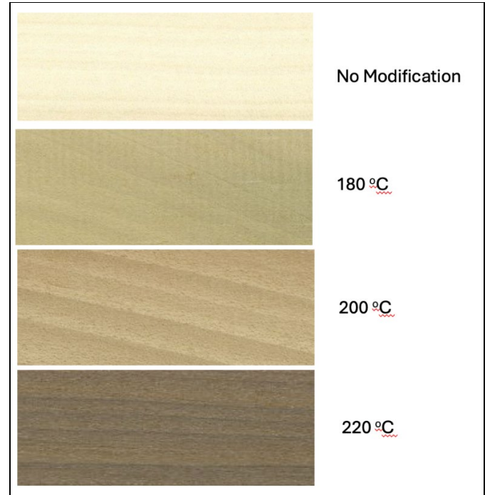
Fig. 1 – Color changes in yellow-poplar at different temperatures during a laboratory test.
