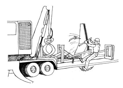
attempted to tighten the binder with a cheater pipe to gain leverage.
